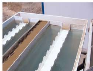
TİKİNER (Lamella) / Thickeners
